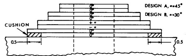
Fig. 6 Composite overlays used to reinforce cutout and cutout-with-crack specimens. Dimensions are in inches (1 in. = 2.54 cm).
